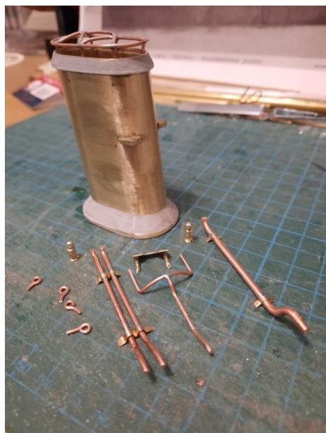
The funnel made from brass and copper wire
