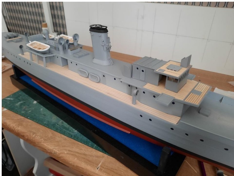
The superstructure taking shape and note the funnel now painted and fitted
