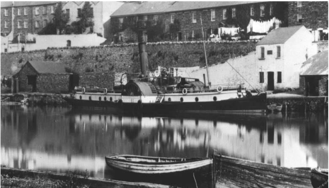
The paddle steamer Alexandrar, pictured here at Calstock, was built by Allsupps, who were well considered builders of small ferries and pleasure steamers. Built in 1888 at 127 tons she sailed from Plymouth on excursion work and had an uneventful career. She was requisitioned in the Great War initially for work delivering market produce from Calstock to Devonport and later for work in Scotland, where she tendered to the Grand Fleet. After the war she returned to excursion work from Plymouth. She was sold in 1927 for scrapping.
