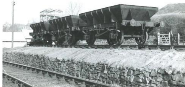
Hopper wagons on the head shunt at Hingston Down Quarry, the main line is in the foreground with the siding rising at 1 in 40
